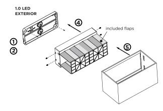
with flaps, the beam angle is adjustable:
